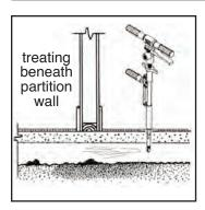
$360^{\circ}$  spray = 2 gal/min  $180^{\circ}$  spray = 2 gal/min
