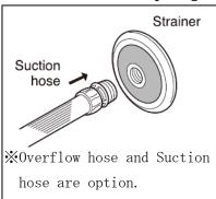
5. Insert the suction hose and overflow hose into the chemical tank.
