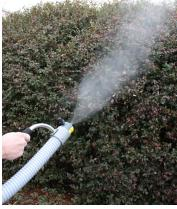
The Versa-Fogger provides a finely atomized fog at a high velocity. It provides good penetration into foliage along with a far reaching fog plume to treat remote areas.
