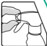
1. When opening, do not hold or pull the trigger. 2. To open, lift up on the nozzle tab and turn the nozzle a quarter turn. 3. To close, turn the nozzle a quarter turn back to the locked position.
