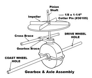
**3.** Install impeller onto pinion shaft. Insert 1/8"x 1½" cotter pin through impeller then through pinion shaft. Use hole closest to the gear box. Spread cotter pin to prevent from falling out. Next insert Cross Brace thru the Gearbox Brace as shown above.
