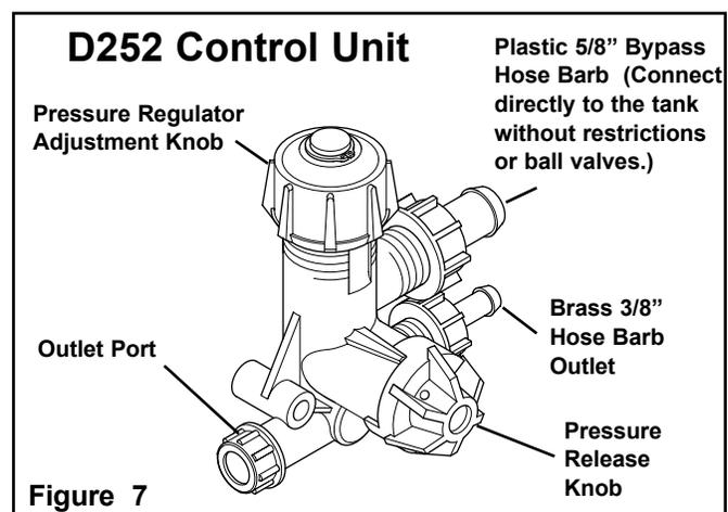
4. The relief valve bypass port should be connected back to the liquid tank without restrictions. Do not hook bypass line back to the inlet port or inlet hose.
