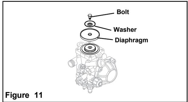
7. Replace the pulsation dampener diaphragm by first bleeding the air from the dampener. Remove the bolts from the dampener cover and replace the diaphragm. Reassemble the cover in place and charge the dampener to 20% of the operating pressure.
